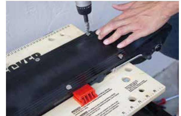
4. Organize the cable, put back the deck and secure the screws. Done.
