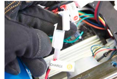
A3. Cut off all the cable ties on the connectors. Disconnect the connectors with the following labels: 1.Load, 5.Display and 6.Charge. Then take out the battery to change another new one.
