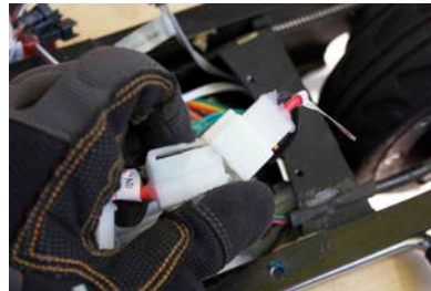
A3. Cut off all the cable ties on the connectors. Disconnect the connectors with the following labels: 1.Load, 5.Display and 6.Charge. Then take out the battery to change another new one.
