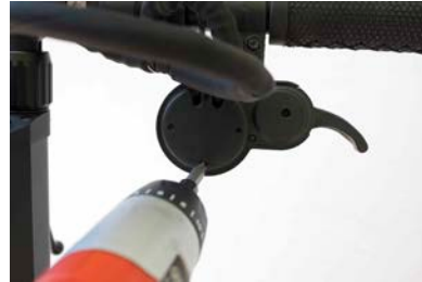
A0. Unscrew and open up the bottom cover of the dashboard and disconnect the 8 pins connector.
