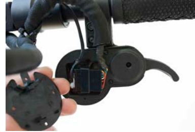
A0. Unscrew and open up the bottom cover of the dashboard and disconnect the 8 pins connector.
