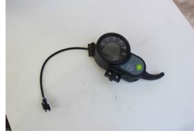
A4. Find out the break bottom signal wire and cut the cable tight.
