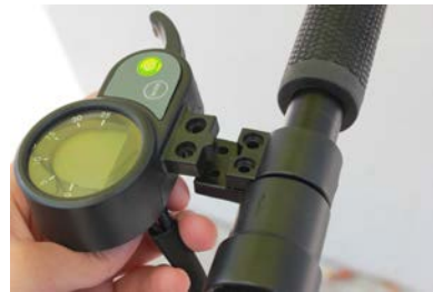
A3. Take the throttle out of the handle.
