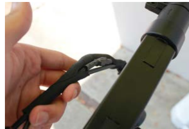
A4. Find out the break bottom signal wire and cut the cable tight.
