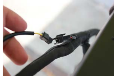
A5. Disconnect the break signal wire, then take out the throttle.
