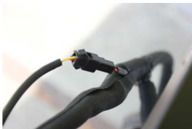
A5. Disconnect the break signal wire, then take out the throttle.
