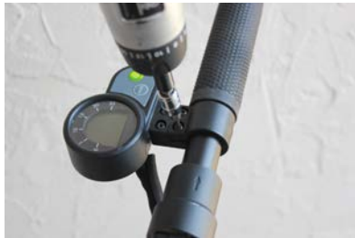
A2. Release the 4 screws on the dashboard.
