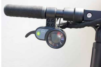
A0. Unscrew and open up the bottom cover of the dashboard and disconnect the 8 pins connector.
