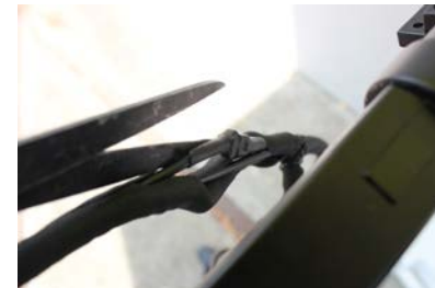
A4. Find out the break bottom signal wire and cut the cable tight.
